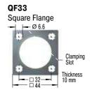
Torque max.: 11 Nm Clamping torque: > 90 Nm Install with 4 machine screws
