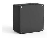
**Description:** Polyester terminal box for increased safety Ex e applications. Compression-moulded glass fibre reinforced polyester with added agents to address static charge build-up. Internal M4 or M6 stainless steel inserts for DIN- and panel-mounting. Mounting location dimensions are moulded into the back side of the enclosure. Covered mounting screw provisions outside of gasketed area.
