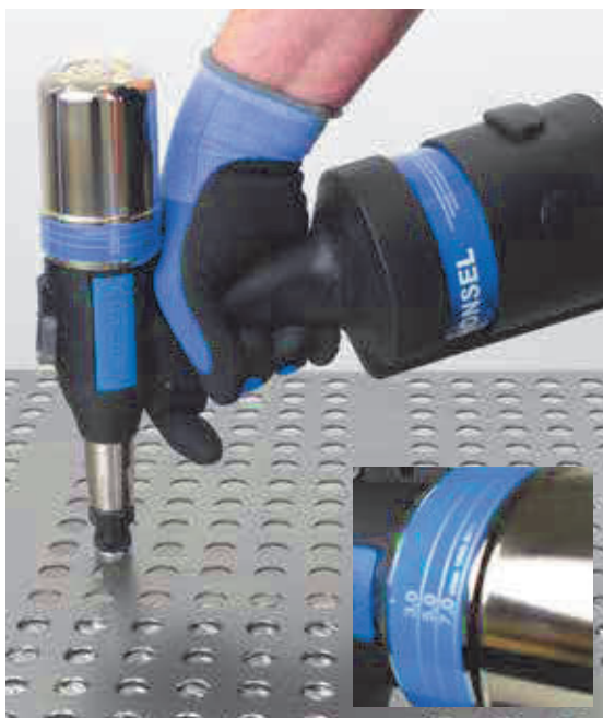
Exact adjustment of the setting stroke via scale on the adjustment cap.
