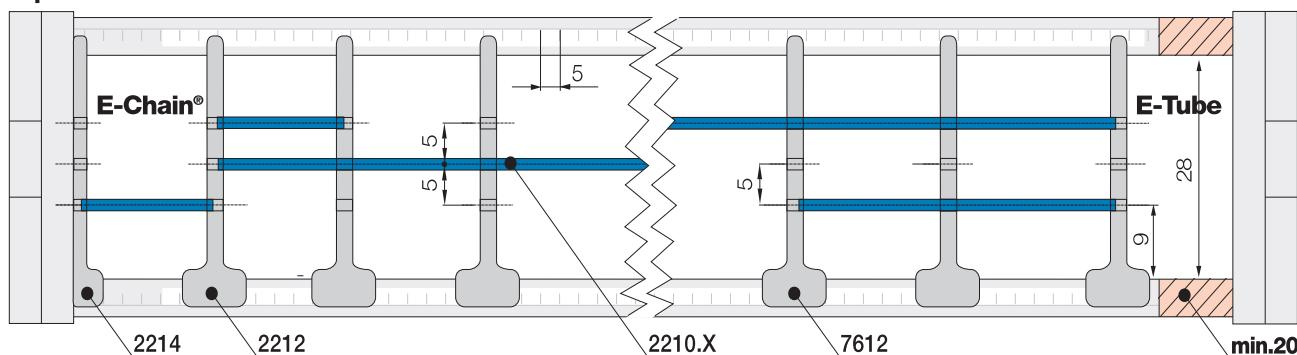
In the standard configuration separators are assembled every 2nd E-Chain® link !
