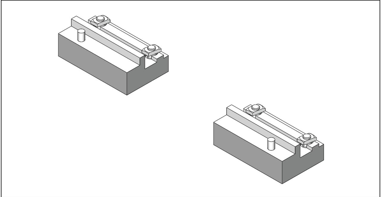
The cross section holder (QSH) is used to attach the cross section element to the main belt element. This is used to convert the height between the main band element (height level 0mm) and the cross-section element (height level +6.7mm).
